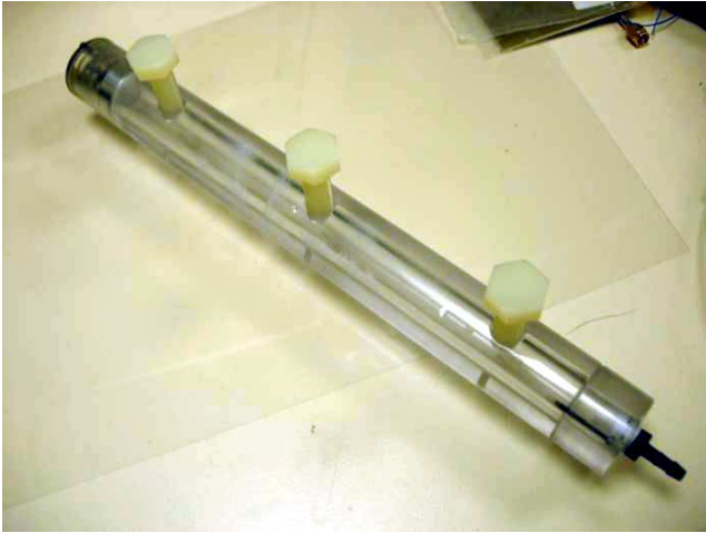
Figure 3: The electrostatic precipitator was machined from perspex, with a piston at the inlet to prevent contamination
