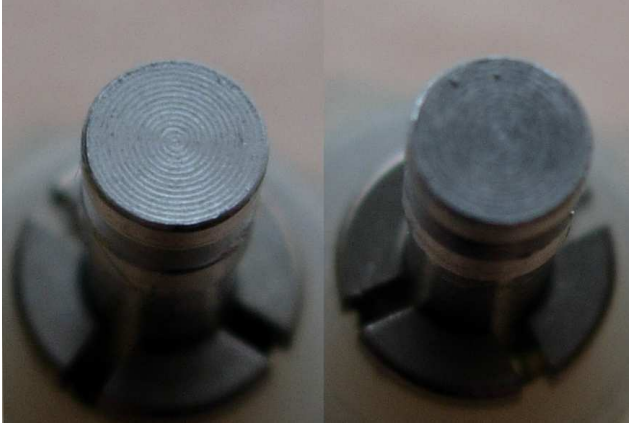
Figure 13: The second and first targets, the second target showing a slight dusting of salt
