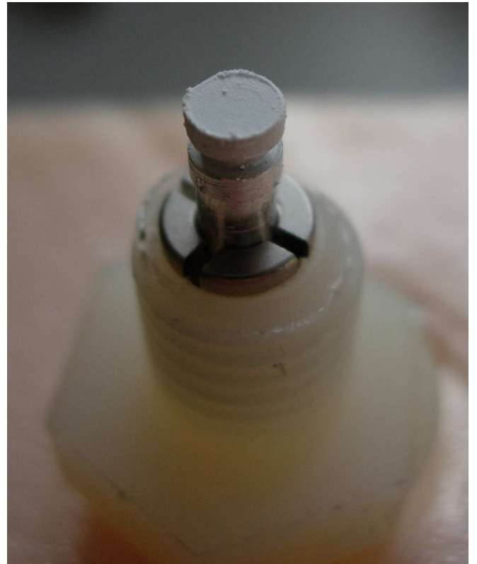
Figure 12: The third SEM target after the test, showing a thick coating of salt
