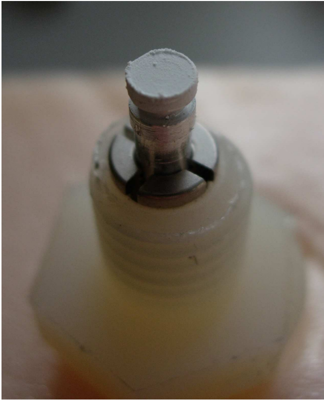
Figure 13: The third SEM target after the test, showing a thick coating of salt
