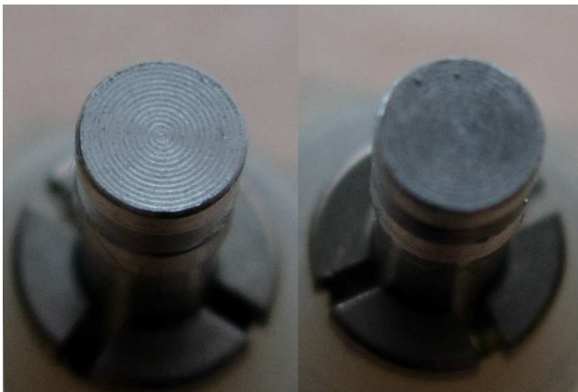
Figure 14: The second and first targets, the second target showing a slight dusting of salt
